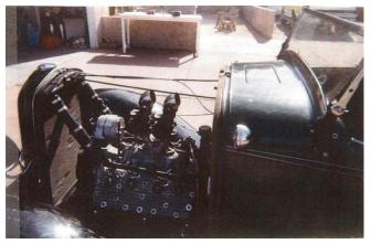
many years of collecting and hoarding of rare parts to complete the engine. The intake manifold is a very early Edelbrock "sling-shot" that had been made in the 1930s. He had two ignitions to choose from. He had a Dynamag magneto that ran on an old stock car that had once competed at the old Dover Speedway and he also had a Kong dual coil ignition that had also run on an old stock car. Anything made by Kong
